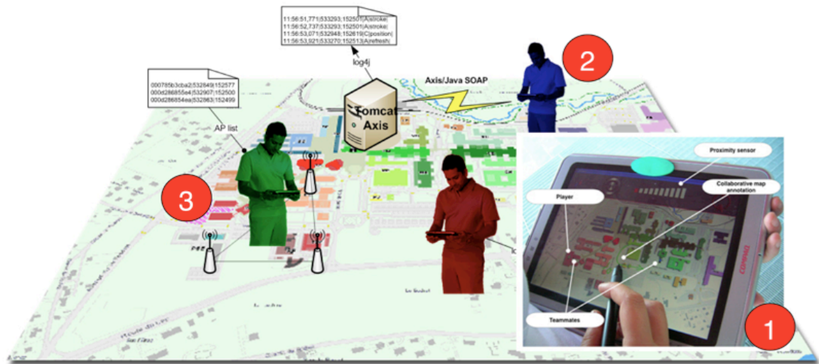
The CatchBob! architecture: (1) Players use TabletPCs to view their and the other players' position. They communicate by annotating the map with a stylus. (2) The data are synchronized over the campus 802.11 network using the SOAP protocol. (3) The positioning algorithm runs on each mobile device. It computes the player's location based on the position of the access points and the signal strength of a radio wave received by the Tablet PCs.
